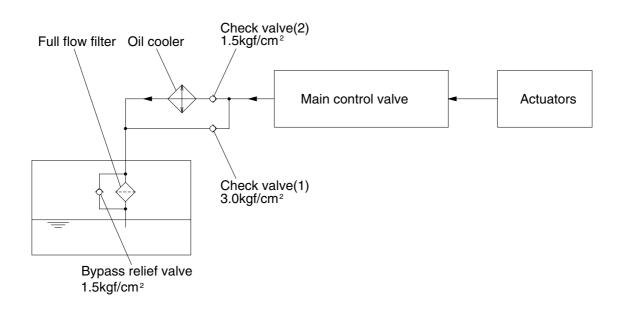
All oil from each actuator returns to the hydraulic tank through the control valve.
