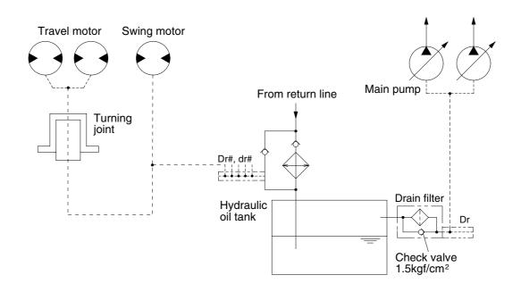
Besides internal leaks from the motors and main pump, the oil for lubrication circulates. These oil have to be fed to the hydraulic tank passing through drain filter.
